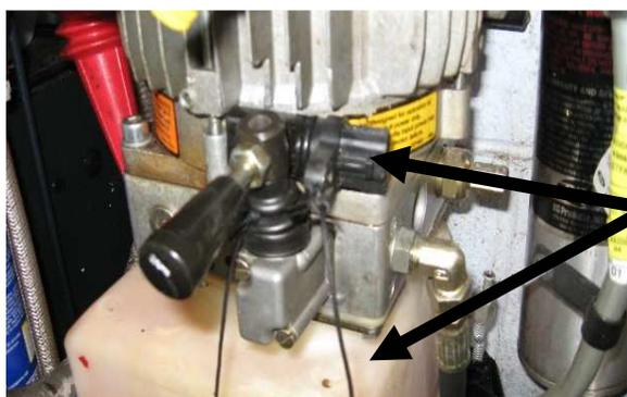
Here is a rotary cassette lift with both the hydraulic controls and safety lock disabled
