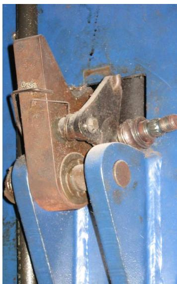
This picture is an example of where the lift safety device has been disabled with what looks like a spark plug.
