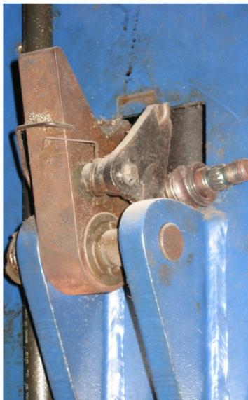
This picture is an example of a lift safety device that has been disabled with what looks like a spark plug.
