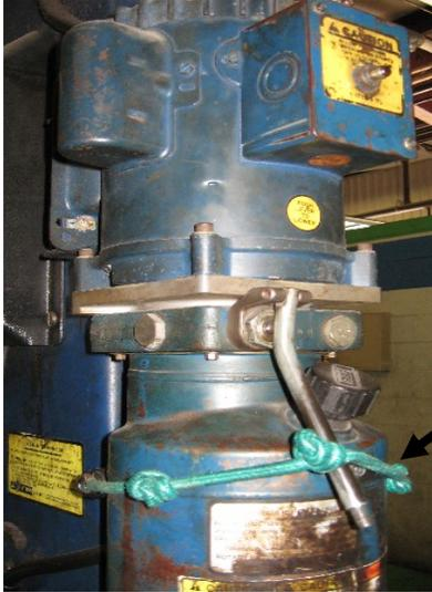
This picture shows how a technician has disabled the hydraulic control lever with a bungee cord to keep the hydraulic controls in an open operating position.
